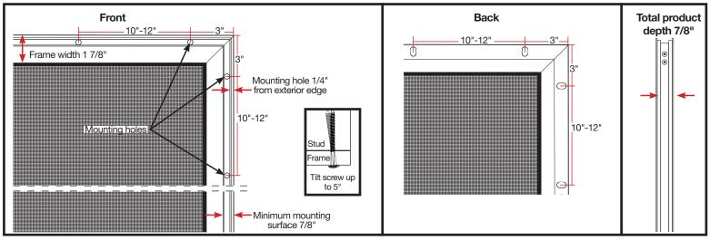
**Quick Escape Ultimate Window Screens** come with pre-drilled mounting holes for surface mount that allow for up to 20 degree screw angle at installation as shown.
