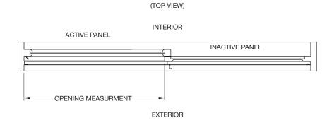
**Note:** Handle height is set at 50-5/8" on-center from bottom mounting surface.
