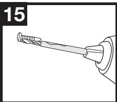
Mark a 1/8" drill bit with tape to indicate the length of the #6-20 x 5/8" self-drilling interlock mounting screw (**I**). Drilling too deeply into the patio door may result in cracked or broken glass.
