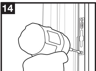
Fasten a latch plate in place using 2 of the #6 x 1/2" flat head self-drilling screws (**M**) provided and remove the tape. Repeat the procedure for the remaining latch plates. Test the operation of the 3-point locking system and adjust latch plate(s) if there is any interference. Slight adjustments to the height of the bottom wheels may also be made to improve lock operation so long as the door continues to slide properly.
