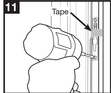
Place the latch plate alignment pin (**H**) on the middle locking knob on the security screen door panel and slide the door closed, moving the adjustable latch plate up or down as needed for the latch plate alignment pin to pass through.
