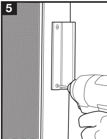
Install the exterior handle (B) on the security screen door panel (A) using the screws (K) provided.
