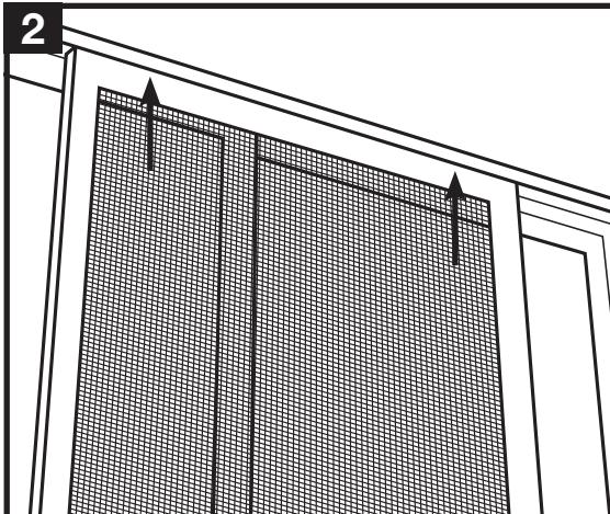
Place the top wheels of the panel (A) into the screen door top pocket, then lift panel up and position the bottom wheels in place on the screen door track.
