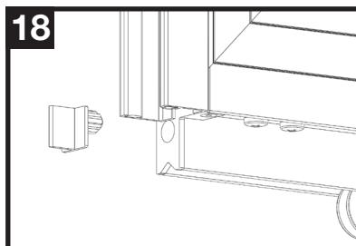
Next insert the round end of the hole plug (**P**) into the adjustment screw hole on the latch side of the door.
