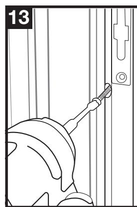
Mark and drill holes to mount the latch jamb extender (**C**) using a 1/8" drill bit. Fasten the latch side jamb extender to the patio door frame using the #6 x 2-1/2" pan head screws (**J**) provided.
