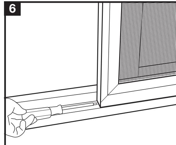
Using the T25 Torx tamperproof security bit (O), adjust the bottom wheels to lift the panel further into the top patio screen door pocket and for smooth sliding operation as needed.
