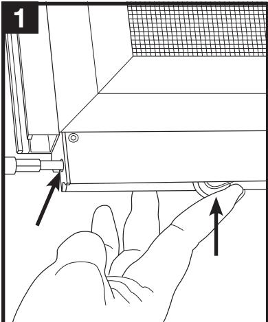
Using the T25 Torx tamperproof security bit (O), adjust the bottom wheels so they are fully retracted.
