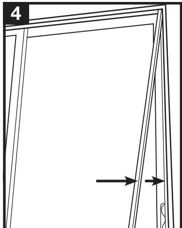
Stand the latch jamb extender (C) in place on the latch side of the main patio door.
