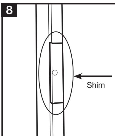
If your main patio door is equipped with a pocket that is deeper than the latch jamb extender mounting leg, attach the shims (G) provided in 5 places on the back of the jamb extender (C) **mounting leg**. It may be necessary to snap together multiple shims to clear the edge of the pocket and install flat in the bottom of the pocket.
