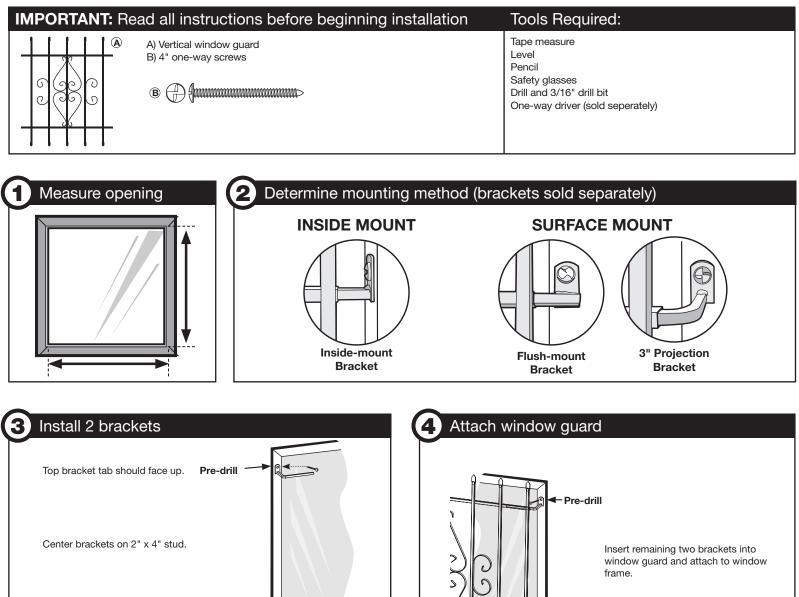
Bottom bracket tab should face down. Pre-drill
