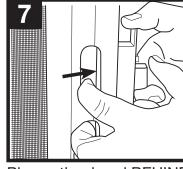
Place other hand BEHIND the black plastic linkage connector and keep pressure on it so that it stays connected to the mortise lock as you pull the mortise lock until it is almost out of the door.
