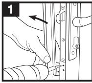
Remove latch guard, if installed (4 mounting screws, 2 top, 2 bottom, on edge of door frame).
