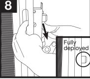
With one hand still keeping pressure on the connector so it remains attached the lock, use the other hand to move the lockset down. Listen for it to click, the top and bottom lock throws will fully deployed.
