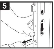
Remove the 2 mortise lock mounting screws in edge of door panel.
