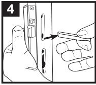
Remove handles and spindle.
