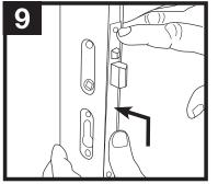
Ensuring the linkage connecter stays attached to the back of the lockset, raise and slide the lockset back into the door panel.
