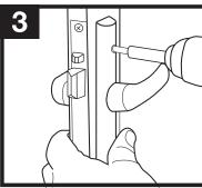
Remove handleset trim plates (2 mounting screws) – hold handles so they do not drop to floor.
