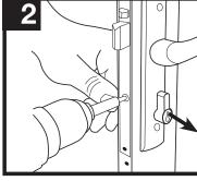
Remove cylinder by removing set screw through edge of door panel and pulling cylinder out of the door.
