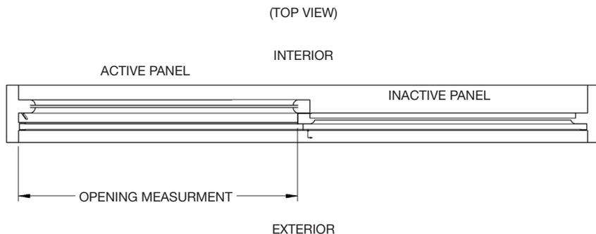
**Note:** Handle height is set at 50-5/8" on-center from bottom mounting surface.
