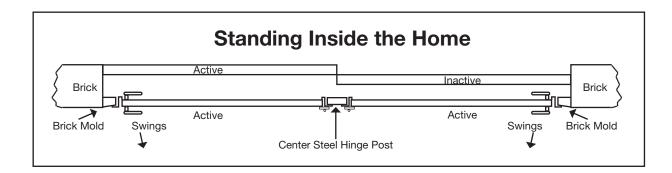
Patio doors will Hinge in the middle, onto a Center Steel Hinge Post and both doors will have a lock on the far outer side jambs, creating a "Butterfly Hinge" system. The Center Steel Hinge Post is not removable and stays in the middle permanently. Because both doors have a lock, you can open them to the clean glass.
