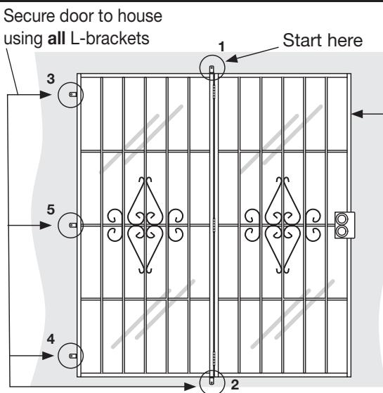
Align this edge of door with edge of mounting surface
