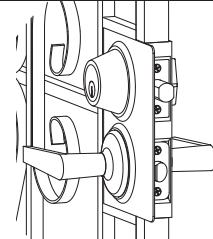
Install your choice of locksets with 2-3/8" backset (sold separately). Fully extend the lock bolts into the "locked" position.
