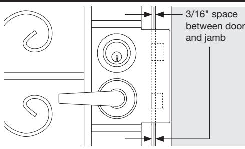
Align the lock bolt holes in the lock-side jamb with the extended lock bolts, allowing approximately 3/16" space between the door and the jamb, from top to bottom. Make sure the jamb is vertically true (plumb).
