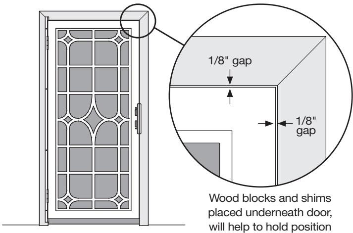
Position door/hinge-side jamb assembly (A) in front of opening. Allow for a 1/8" gap between the lock-side edge of door and inside-edge of your mounting surface, as well as a 1/8" gap between the top-edge of door and bottom-edge of your mounting surface (see illustration).
