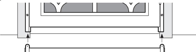
Place bottom bar (**D**) beneath the side jambs. Both ends should reach the outer edge of the side jambs. Hold in place and use 5/32" drill bit to pre-drill holes for mounting screws. Attach bottom bar to each side jamb using the provided screws (**H**).
