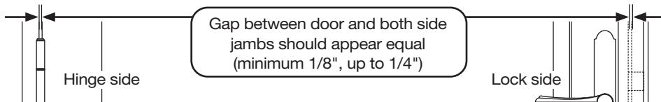
Align the lock holes in the lock-side jamb with the lock bolts extended. Maintain a space between door (A) and the lock-side jamb (B) equal or similar to the space between the door and hinge-side jamb, from top to bottom. Making sure the lock-side jamb is plumb, mark the location of the mounting holes. Set the jamb aside and, where marked, pre-drill 3/16" holes. Return jamb to position and fasten to house using the provided one-way screws (G).
