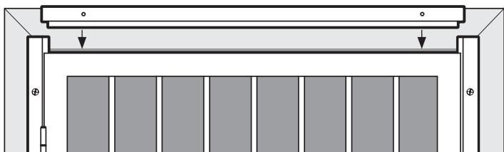
Place the top header jamb (**C**) above the door and between the two side jambs. Spacing should be equal, from left to right, above the door and be similar to spacing determined in **Step 2**. Mark the location of the mounting holes. Set the jamb aside and, where marked, pre-drill 3/16" holes. Return jamb to position and fasten to house using the provided one-way screws (**G**).
