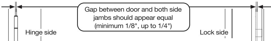
Align the lock holes in the lock-side jamb with the lock bolts extended. Maintain a space between door (A) and the lock-side jamb (B) equal or similar to the space between the door and hinge-side jamb, from top to bottom. Making sure the lock-side jamb is plumb, mark the location of the mounting holes. Set the jamb aside and, where marked, pre-drill 3/16" holes. Return jamb to position and fasten to house using the provided one-way screws (G).
