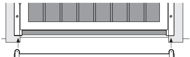
Place bottom bar (**D**) beneath the side jambs. Both ends should reach the outer edge of the side jambs. Hold in place and use 5/32" drill bit to pre-drill holes for mounting screws. Attach bottom bar to each side jamb using the provided screws (**H**).
