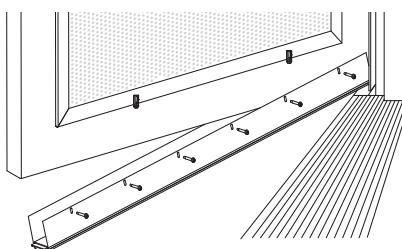
Open the door. Slip the multi-blade bug sweep (**F**) onto the bottom of the door. Hold sweep in place and close the door. Allow the sweep to fall and set rested on the threshold plate (**E**).
