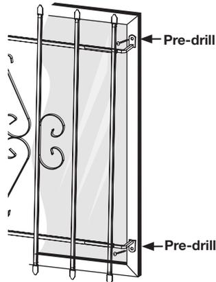
Insert remaining two brackets into window guard and attach to window frame.
