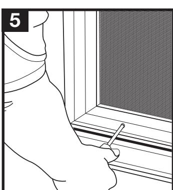
Test the slide of both doors. Using a phillips-head screw driver adjust bottom wheels up or down if necessary for optimum slide.
